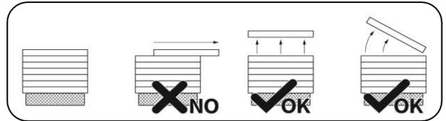
If necessary, depending on the size and weight of the individual panel, it is advisable to provide suitable mechanical lifting devices, such as **suction cup lifters** or special **grippers/jaw clamps**.
